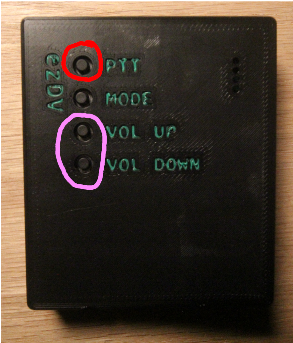
Figure 5: ezDV showing the PTT button (red circle) and the Volume Up/Down buttons (pink circle)
