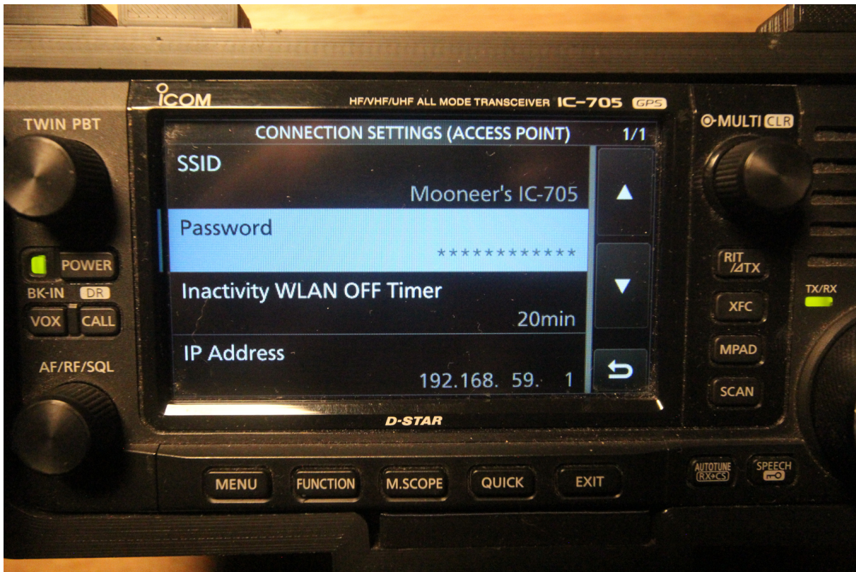
Figure 33: Icom IC-705 displaying Access Point settings
