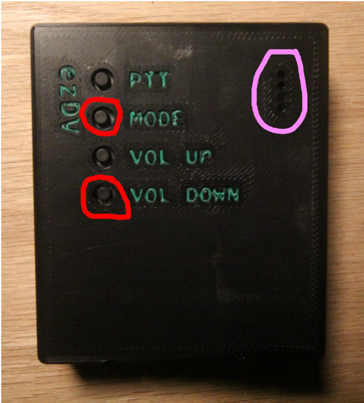
Figure 3: ezDV showing the buttons to push and hold (red circles) and the location of the LEDs (pink circle)
