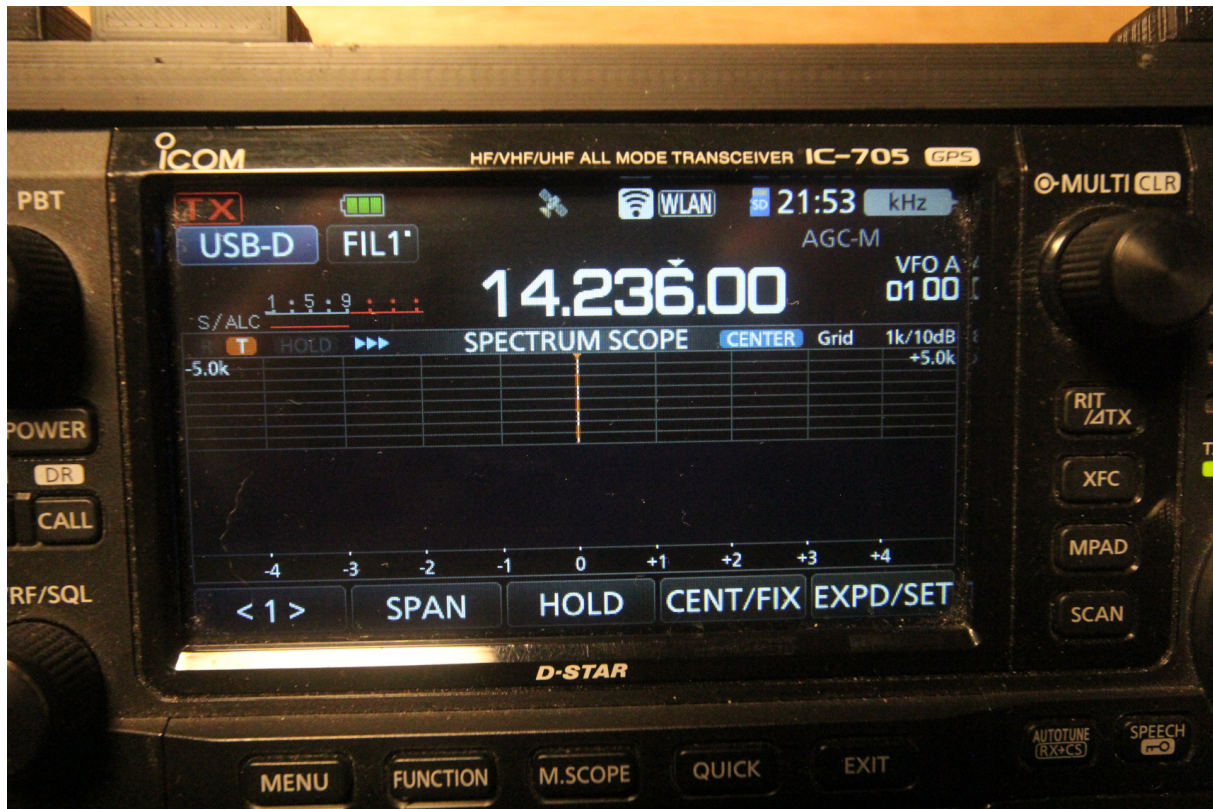
Figure 10: Icom IC-705 properly connected to ezDV (WLAN indicator at the top of the screen)
